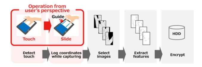
Figure 2: How the new technology is used, and how it processes information. Credit: Fujitsu
