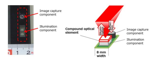
Figure 1: Prototype optical unit. (Left, photo: a dotted line surrounds the components; right, a schematic diagram). Credit: Fujitsu
