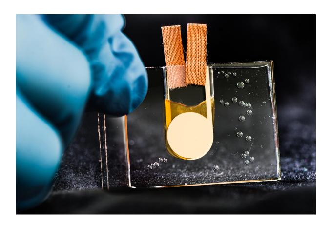
Heat driven transistor on Laboratory of organic electronics, Linköping University. Credit: Thor Balkhed
