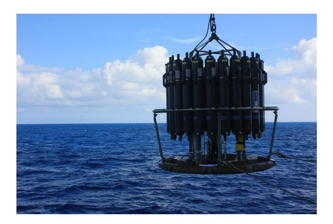
An oceanographic sampler, known as a rosette, during a 2013 cruise in the North Pacific. Each bottle contains water from different depths, which is how researchers collected samples of the vitamins at sea. Credit: Kevin Simans/University of Washington
