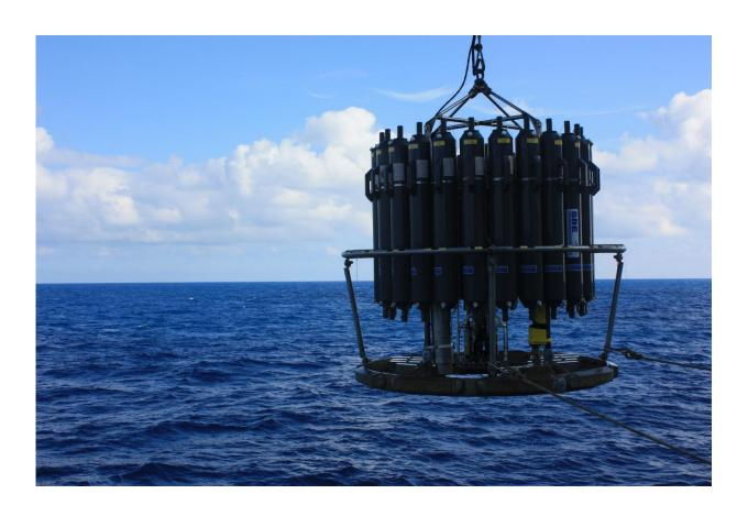
An oceanographic sampler, known as a rosette, during a 2013 cruise in the North Pacific. Each bottle contains water from different depths, which is how researchers collected samples of the vitamins at sea. Credit: Kevin Simans/University of Washington
