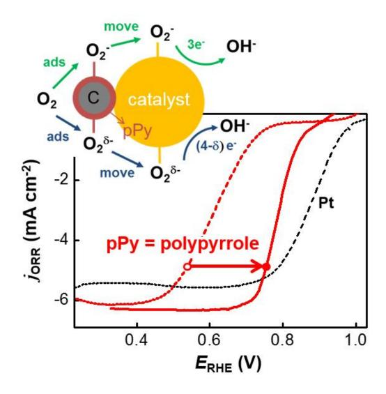
The oxygen reduction reaction at the anode of the cell is divided into four stages. The first step, which is the slowest, involves the addition of polypyrol to improve the catalytic reaction. Credit: UNIST
