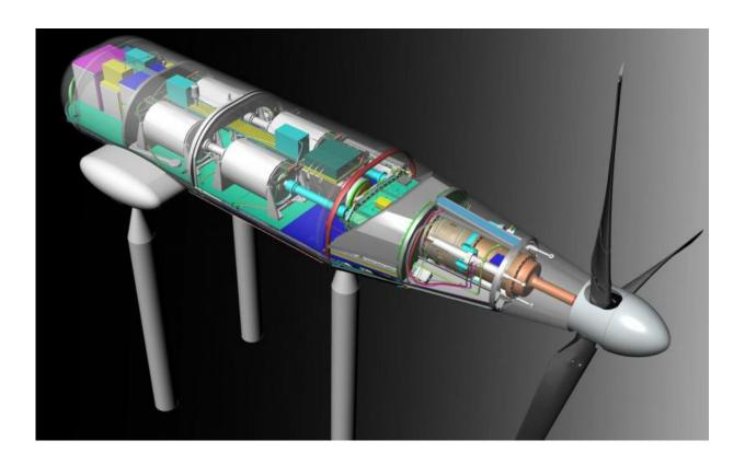
Design concept for the TTR, showing internal components of the control system, motors and gearbox. Credit: NASA
