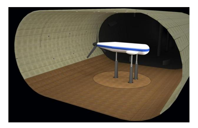
This computer rendering shows the TTR once installed in the huge wind tunnel. Credit: NASA
