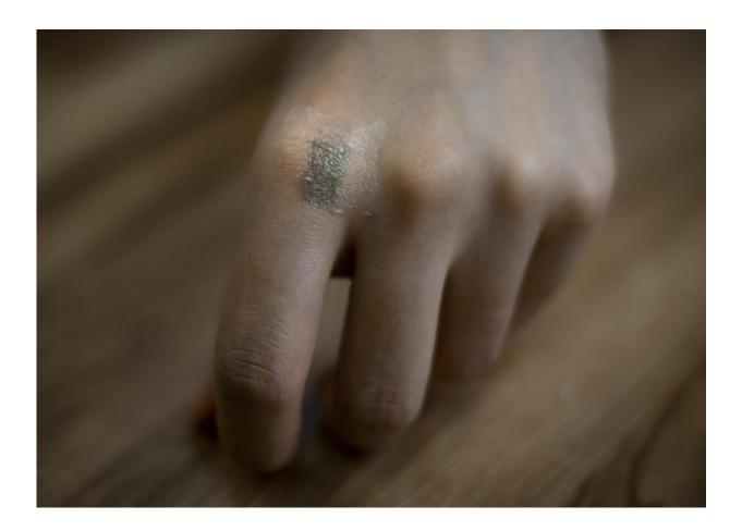
Fully stretchable transistor as a secondary e-skin on hand knuckle. Credit: Jie Xu, Sihong Wang
