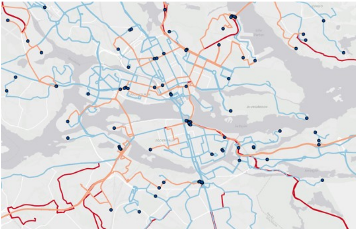
A map of bus lines in Stockholm showing where electrical lines with wireless charging would be possible. The red lines represent biodiesel, blue lines represent electrical / conductive charging and orange lines electric / inductive charging. Credit: KTH Royal Institute of Technology
