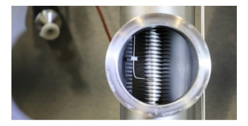
Heat exchangers from instant water heaters provided the solution: the sodium hydroxide solution spirals along a pipe, absorbs water vapor and emits heat. Credit: Swiss Federal Laboratories for Materials Science and Technology
