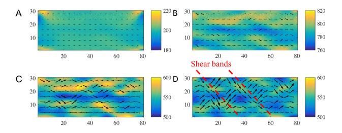
Predictions of various deformation fields in the Vitreloy 1 simulation created at Rice University at various stages of deformation and with an ambient temperature of 698 degrees Fahrenheit. Each plot shows the equivalent stress overlaid with the strain field. The color bar on the right of each plot shows the magnitude of the stress in units of megapascals. Credit: Apiwat Wisitsorasak/King Mongkut University of Technology
