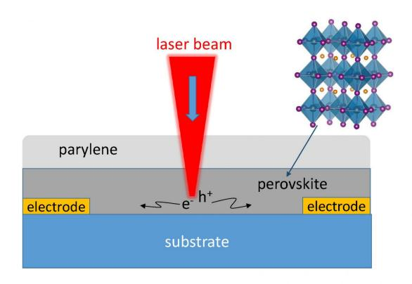
This is a schematic of scanning photocurrent imaging microscopy of halide perovskite film (side view). Using the technique, researchers found the diffusion length within a well-oriented perovskite film measured up to 20 micrometers. Credit: *Nano Letters*
