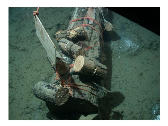
Freshly deployed log in the Norwegian Sea. For each experiment, one large log as well as several smaller ones were deposited on the sea floor with the help of an remotely operated vehicle. Credit: Marum, University of Bremen
