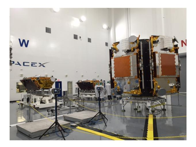
IridiumNEXT satellites being fueled, pressurized & stacked on dispenser tiers at Vandenberg AFB for Falcon 9 launch. Credit: Iridium
