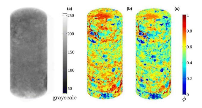
X-ray tomography images of soil cores pinpoint the concentrations of solids (left, in grey) and the distribution of solids and pores (right, in color). Credit: Pacific Northwest National Laboratory
