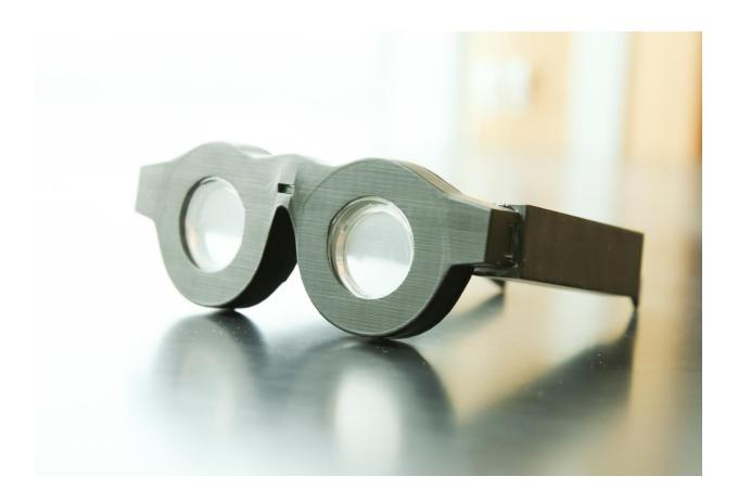
Early prototype of 'smart glasses' with liquid-based lenses that can automatically adjust the focus on what a person is seeing, whether it is far away or close up. The lenses are placed in battery-powered frames that can automatically adjust the focal length of the lenses based on what the wearer is looking at. Researchers expect to have smaller, lighter frames with the technology in as early as three years. Credit: Dan Hixson/University of Utah College of Engineering
