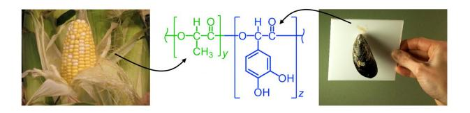
Purdue University researchers have developed a new type of adhesive that combines the bonding chemistry of shellfish with a bio-based polymer that can be derived from corn. This adhesive was created by harnessing the chemistry of compounds called catechols, represented in the blue portion of the chemical formula in this graphic. Credit: Purdue University photo/Jonathan Wilker
