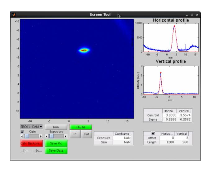
The bright red spot on this display shows the passage of the first beam to circulate in the SESAME main ring. Credit: SESAME
