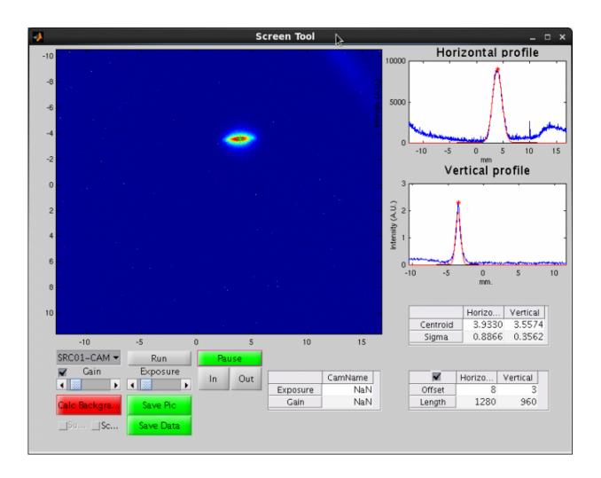
The bright red spot on this display shows the passage of the first beam to circulate in the SESAME main ring. Credit: SESAME
