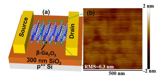
The schematic at left shows the design for an experimental transistor made of a semiconductor called beta gallium oxide, which could bring new ultra-efficient switches for applications such as the power grid, military ships and aircraft. At right is an atomic force microscope image of the semiconductor. Credit: Purdue University image/Peide Ye
