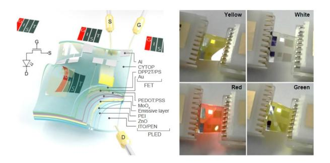
Field-effect transistors integrated with LEDs, showing transparency and
