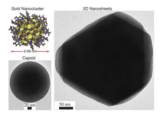
2D hexagonal sheet-like and 3D capsid structures based on atomically precise gold nanoclusters as guided by hydrogen bonding between the ligands. The inset in the top left corner shows the atomic structure of one gold nanocluster. Credit: Academy of Finland
