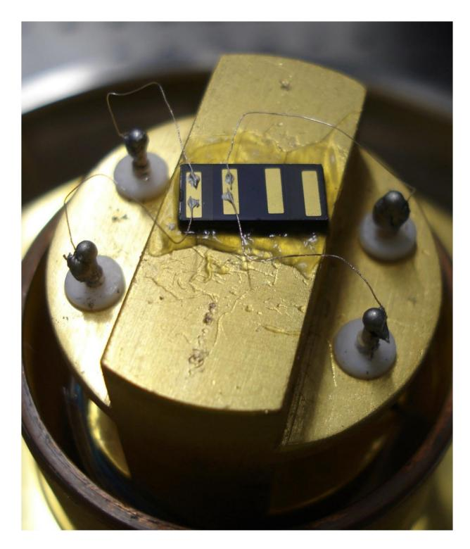
The experimental polaron solar cell in the lab. Credit: Dirk Raiser, MPIbC/DESY
