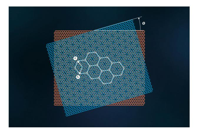
Fig. 2. The third type of bigraphene known as twisted bilayer graphene. The white hexagons mark the boundaries of superlattice cells (moiré pattern cells). Credit: MIPT Press Office
