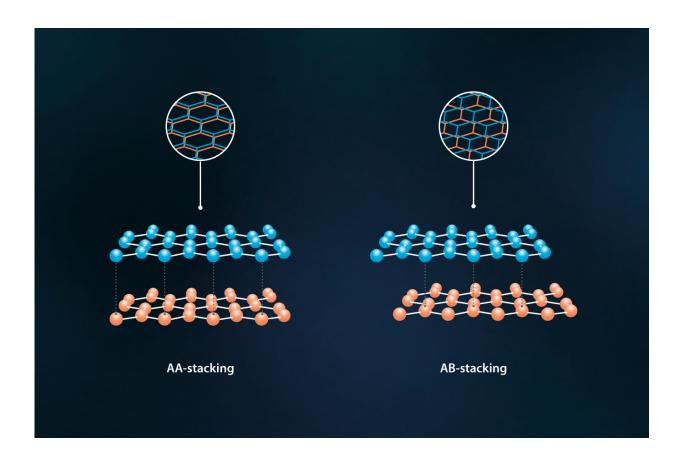
Fig. 1. Two types of bigraphene: AA-stacked bilayer graphene where each atom in the upper sheet sits exactly on top of an atom in the lower sheet and ABstacked bilayer graphene where only half of the atoms in the upper sheet lie over another atom, whereas the other half lie over the center of a hexagon formed by the atoms in the lower sheet. Credit: MIPT Press Office
