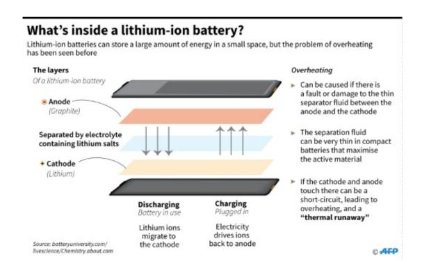
The basic components of lithium-ion batteries, and how they can overheat
