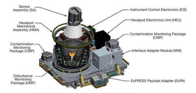
This graphic illustrates the components that make up the SAGE III Instrument Payload. Credit: NASA
