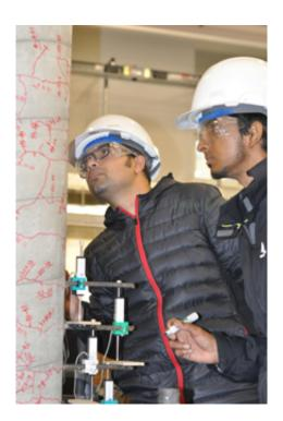
Test leader Mosharef Hossain, right, along with fellow UBC engineering student Rashedul Kabir, left, carefully inspect a concrete column after it has been put through a lengthy shake test at UBC Okanagan's Applied Laboratory for Advanced Materials and Structures. Credit: UBC Okanagan
