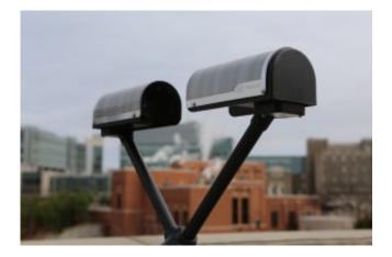
A laser beam passing between the two heads of the distrometer detects the numbers and sizes of passing raindrops or snowflakes. Credit: Duke University
