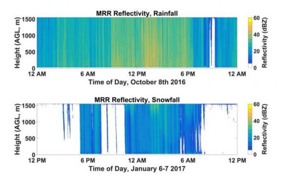
The Micro Rain Radar (MRR) shoots radio waves into the sky where they reflect off water droplets or snowflakes, revealing the size and height of clouds or precipitation. The team collected continuous MRR data during Hurricane Matthew (top) and last Friday's snow storm (bottom), creating these colorful plots that illustrate precipitation rates during the storms. Credit: Duke University
