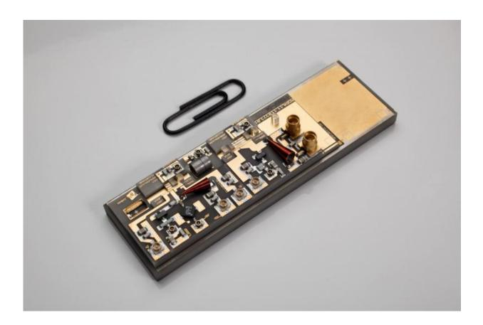
Hybrid-integrated master-oscillator power-amplifier (MOPA) laser module for rubidium precision spectroscopy in space developed by the Ferdinand-Braun-Institut – three of these MOPA modules along with two redundant modules are integrated into the laser system. Credit: FBH/schurian.com
