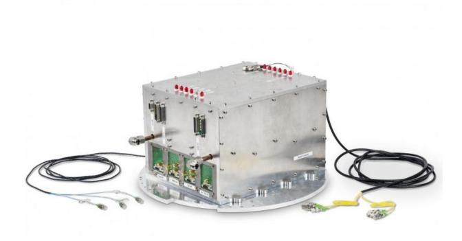
MAIUS laser system used to successfully create a Bose-Einstein condensate for the first time in space. It is about as big as a shoe box with a mass of 27 kg. FBH's laser modules are integrated on the bottom side of the heat sink, the top side houses modules for further processing of the light to be transferred to the main experiment. Credit: Humboldt-Universität zu Berlin
