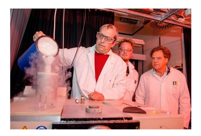
The research team Carsten Kötting, Daniel Mann and Klaus Gerwert (left to right) sets up the measuring equipment. The detector of the spectrometer has to be cooled with liquid nitrogen. Credit: RUB, Marquard
