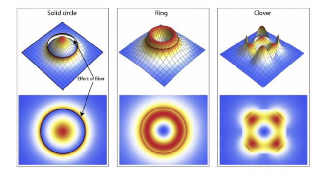
Examples of light shapes. Each panel shows a 3D (top) and 2D (bottom) intensity profile. The red (blue) areas indicate more (less) light intensity. The effect of the fiber appears in the 3D images as a sharp cutout; in 2D the fiber interface looks like a ring-shaped edge. Credit: P. Solano and L. Orozco
