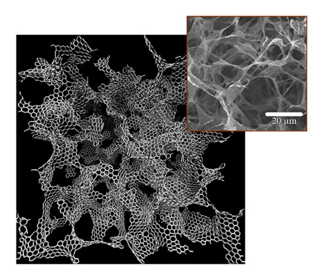
A three-dimensional graphene assembly and scanning electron microscope image
