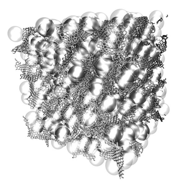
The closely packed graphene-inclusion structure obtained after cyclic equilibrations. Credit:Qin et al. Sci. Adv. 2017;3:e1601536
