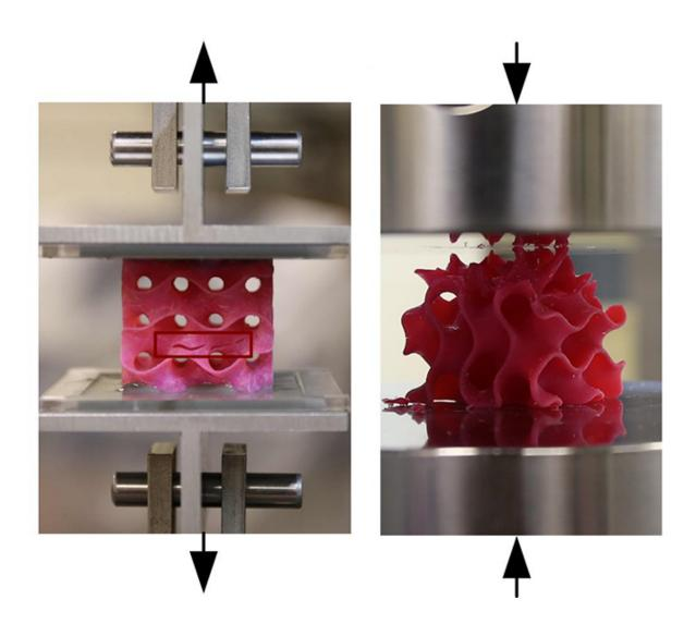
Tensile and compressive tests on the printed sample. Credit: Qin et al. Sci. Adv. 2017;3:e1601536
