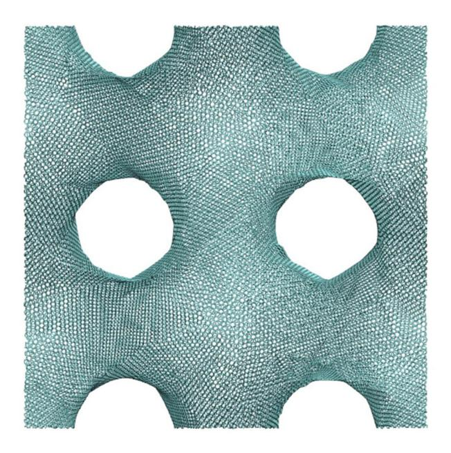
Model of gyroid graphene with 20 nm length constant. Credit: Qin et al. Sci. Adv. 2017;3:e1601536
