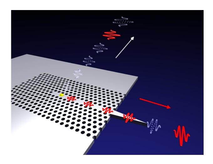
Illustration of a photon gun. A quantum dot (the yellow symbol) emits one photon (red wave packet) at a time. The quantum dot is embedded in a photonic crystal structure, which is obtained by etching holes (black circles) in a semiconductor material. Due to the holes, the photons cannot be emitted in all directions, but only along the waveguide, which is formed by omitting a number of holes. Credit: Søren Stobbe, NBI
