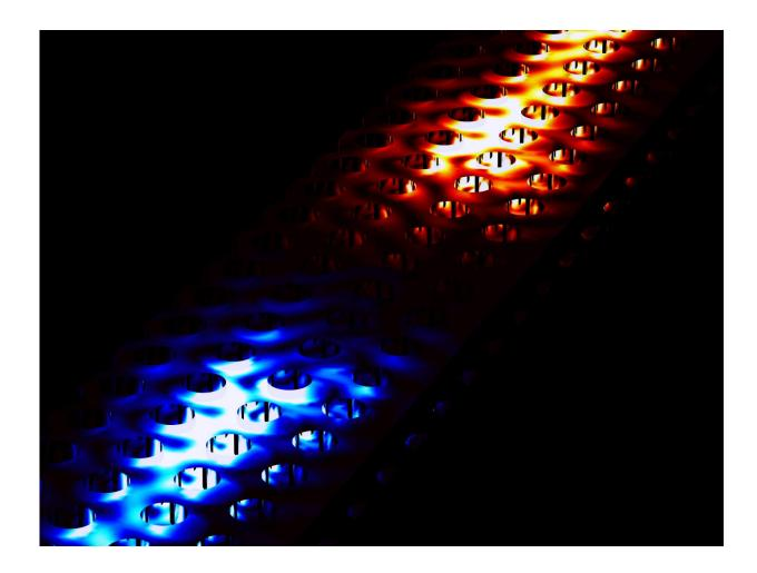
Directional emission of photons. The figure shows the calculations of the photon emission in the new directional single-photon source. If the spin of the quantum dot's electron points up, the photon will be emitted in the one direction (blue). If the spin of the quantum dot's electron points down, the photon will be emitted in the opposite direction (red). Credit: Sahand Mahmoodian and Søren Stobbe, NBI
