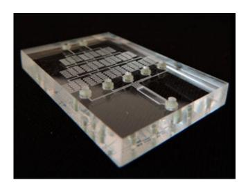
A microfluidic device made by A\*STAR scientists for on-the-spot blood analysis. Credit: A\*STAR Singapore Institute of Manufacturing Technology
