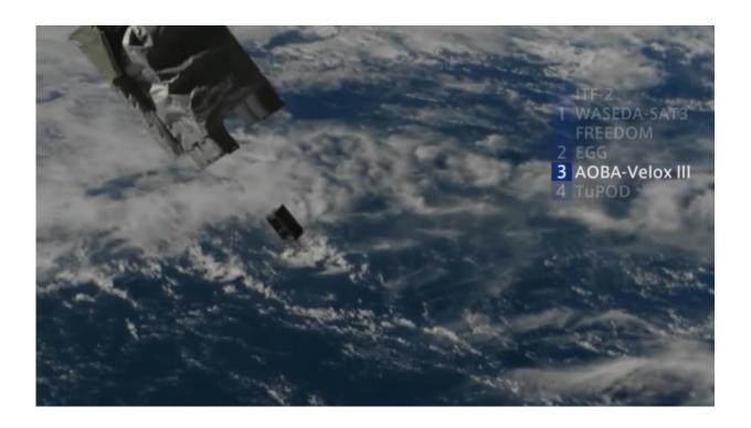
The ISS new JEM Small Satellite Orbital Deployer is on the upper left, which is seen launching out the AOBA-VELOX III using springs. Credit: JAXA
