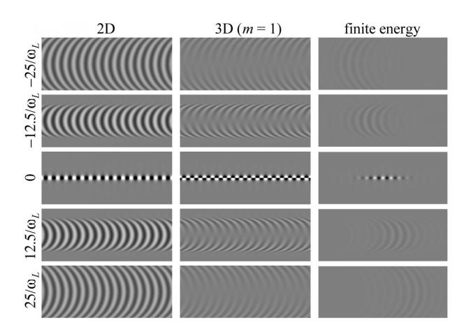
Three representations of the 'needle pulse' beam, showing how the circular wave fronts collapse into a needle-like thin power distribution with no side lobes. Credit: Kevin Parker/Miguel Alonso
