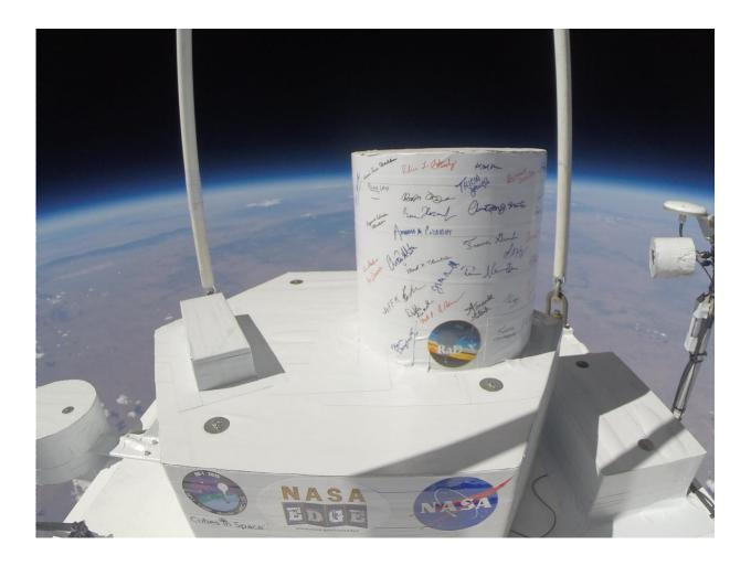
The RaD-X payload ascended into the stratosphere to measure cosmic radiation coming from the sun and interstellar space. Credit: NASA
