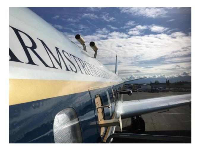
As the DC-8 flies, these inlets collect air into the more than 20 scientific instruments aboard, which measure various atmospheric gases and pollutants. Credit: NASA/Roisin Commane
