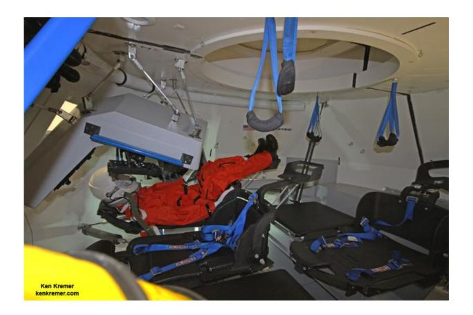
Looking inside the newly upgraded Starliner mockup with display panel, astronauts seats, gear and hatch at top that will dock to the new International Docking Adapter (IDA) on the ISS. Credit: Ken Kremer/kenkremer.com
