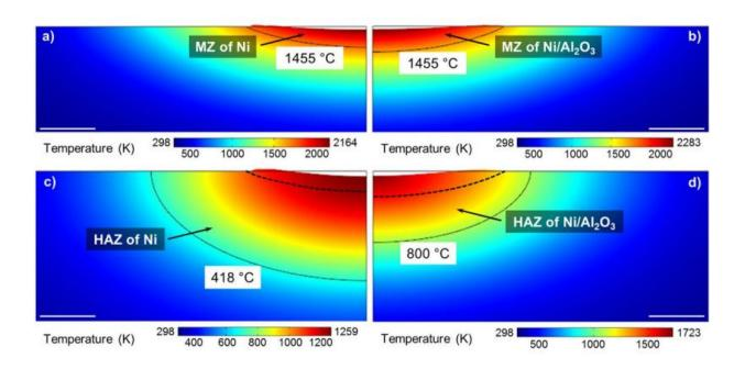
Adding nanoscale particles of aluminum oxide increases the depth of the melting zone (MZ) in nickel and decreases the size of the heat-affected zone (HAZ). The bottom right image shows how even at higher temperatures the heat affected zone doesn't grow very large. Credit: UCLA Engineering
