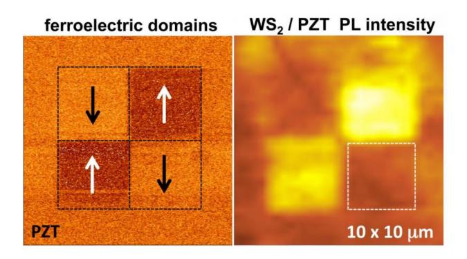
Domains consisting of electric polarization dipoles are written in a checkerboard pattern into a thin film of lead zirconium titanate (PZT) with a conductive atomic force microscope, and imaged with the same instrument (left panel). Both intensity and spectral distribution of the photoluminescence emitted from a monolayer of tungsten disulphide (WS2) transferred onto the PZT surface is strongly modulated by these polarization domains (right panel). Credit: U.S. Naval Research Laboratory
