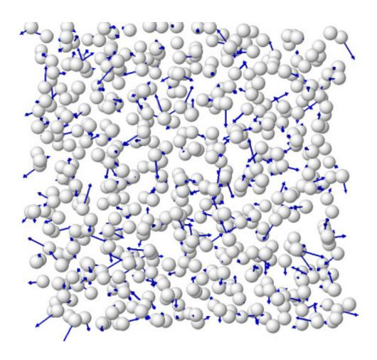
Asegun Henry and his group at Georgia Tech have developed a new formalism called the Green-Kubo Modal Analysis (GKMA) method that allows one to calculate the modal contributions to thermal conductivity for any material or object where the atoms vibrate around equilibrium sites. They are currently applying the method to amorphous materials like glass. Credit: Asegun Henry, Georgia Tech
