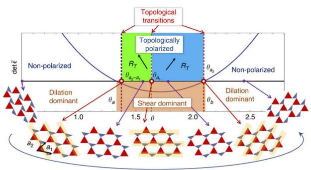
Transforming lattice with uniform soft twisting  $\theta$
