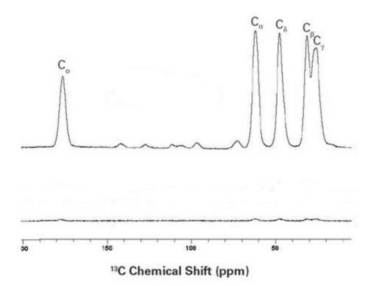
In this specific case, the EPR signal is seventy times stronger with the use of an amplifying agent, like the researched AMUPol (top), than without (bottom). Credit: Leiden Institute of Physics
