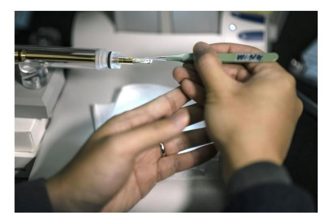
Purdue postdoctoral research associate Jie Jian mounts a ceramic sample for research using a transmission electron microscope. The work is related to ceramics manufacturing for various military and commercial uses. Credit: Purdue University image/Erin Easterling
