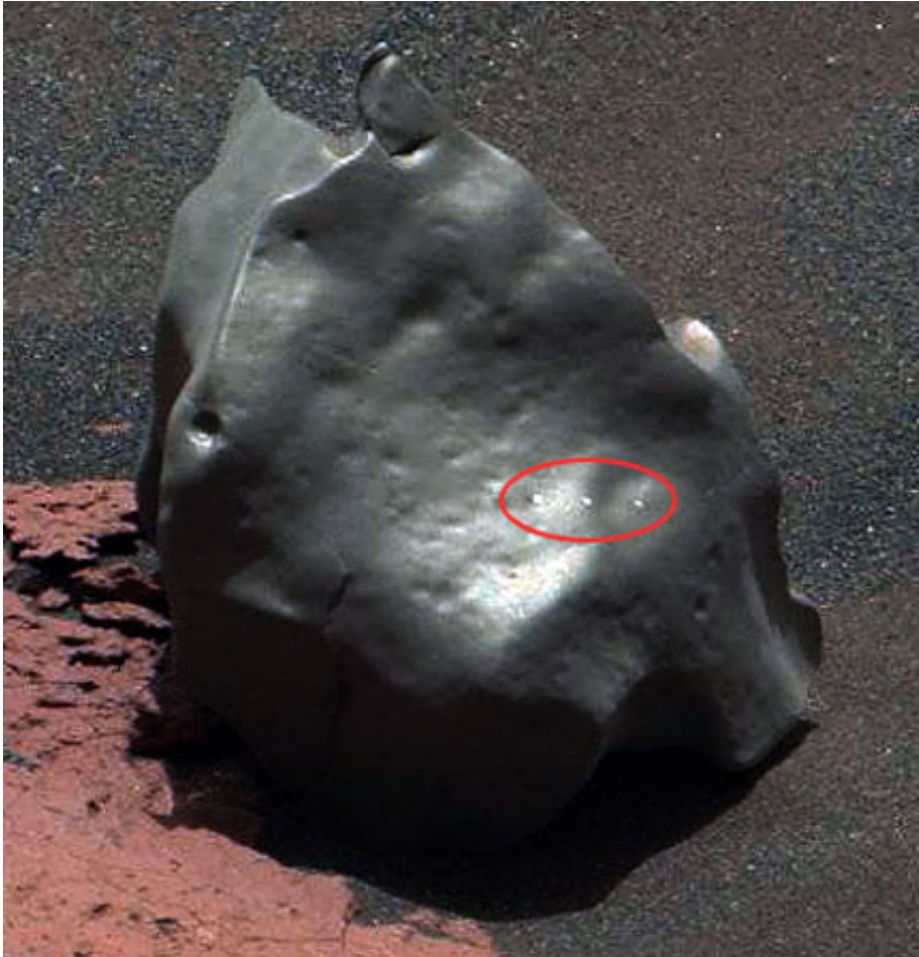
Closeup showing laser zap pits. Credit: NASA/JPL-Caltech/MSSS
