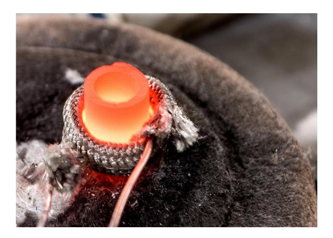
Researchers have developed a new low-cost technique for converting bulk powders directly to oxide nanowires. Shown is a crucible in which an alloy of lithium and aluminum is being formed. Credit: Rob Felt, Georgia Tech
