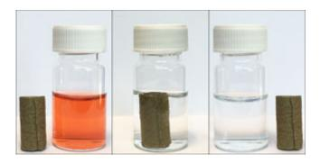
Iron-based coatings with elongated nanoscale 'fins' can easily absorb large amounts of dye molecules from contaminated water. Credit: The Royal Society of Chemistry
