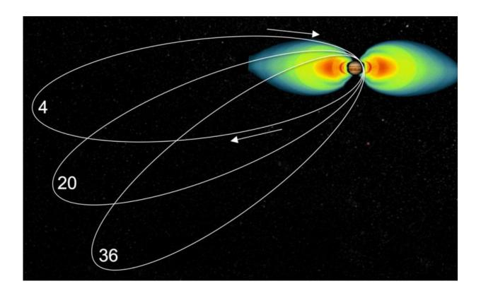
The tilt of Juno's orbit relative to Jupiter changes over the course of the mission, sending the spacecraft increasingly deeper into the planet's intense radiation belts. Orbits are numbered from early in the mission to late. Credit: NASA/JPL-Caltech
