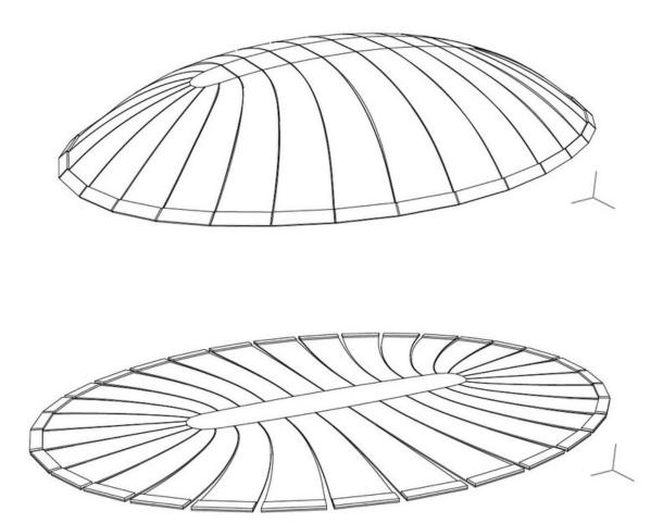
Geometry optimized dome and unrolled initially flat slab before inflation. Credit: Geometry optimization DI Thomas Pachner
