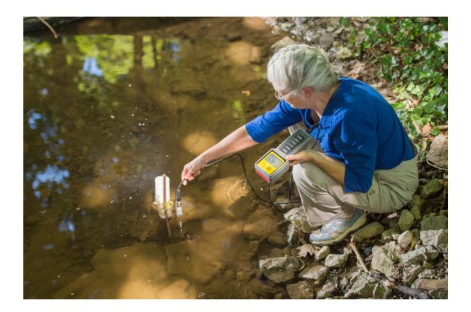
Pam Silver takes a reading from Glenhill Stream on the Behrend campus. The white device in the water is a data logger that records conductivity and temperature of the water every 15 minutes. Because Silver downloads data from the logger just once a year, she takes readings monthly with a hand-held unit. Credit: Robert Frank
