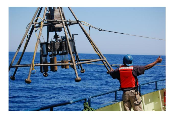
The multicorer device being lowered into the ocean takes eight one-foot cores from the seafloor. Scientists analyze such cores for clues to the climate of the past several thousand years. Credit: Peter deMenocal
