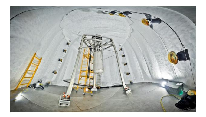
The Large Underground Xenon experiment installed 4,850 ft underground inside
